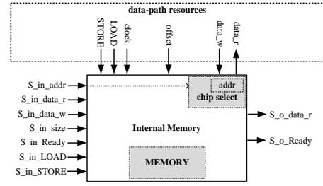
Figure 6: Structure of the interface with an internal memory.
