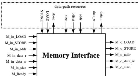
Figure 5: Structure of the interface to the external memory.
