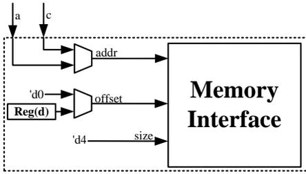
**Figure 12: Resulting connections to the memory interface for the function bar.**  $Reg(d)$  represents the out port of the register where the variable  $d$  is stored.
