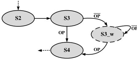
Figure 4: Example of FSM with an unbounded operation in S3. The input  $OP$  represents that the *done* signal has been received, while  $\overline{OP}$  means that the controller is still waiting for the same signal. S3\_w is the waiting state associated with S3.
